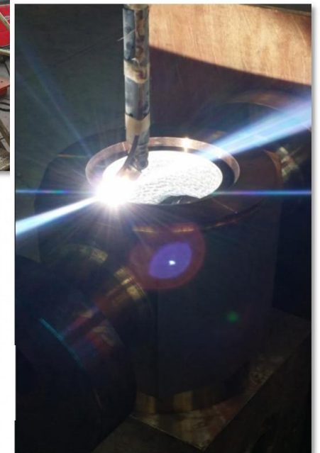
The valve body is welded with a 625-nickel-based alloy.
